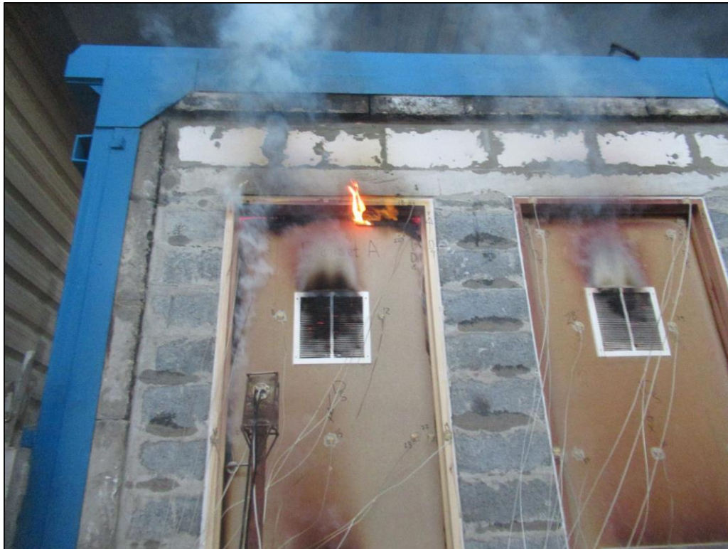
Picture 9: Sustained flaming for more than 10 seconds was observed on the top horizontal edge of door A leaf at 46:30 minutes, causing the integrity failure of doorset A. The doorset was then covered with a gypsum board, and the test was continued further for doorset B only.
