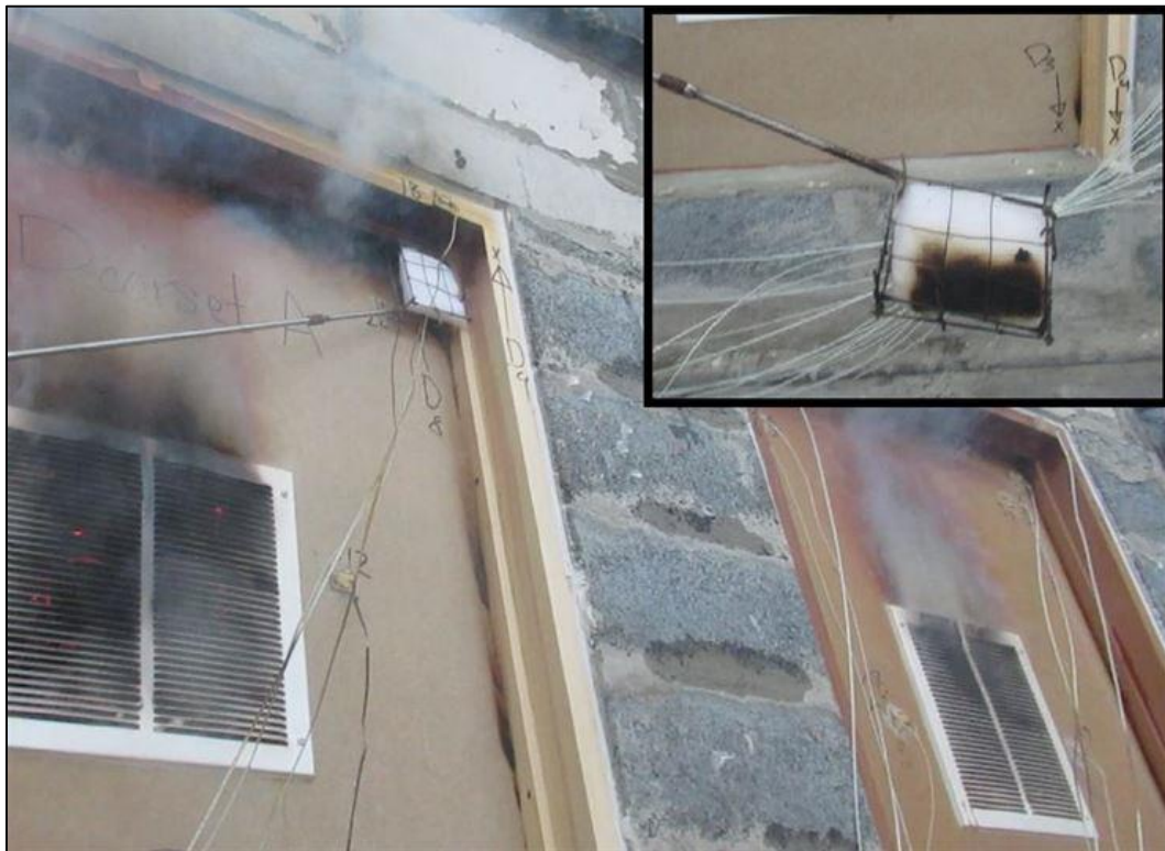
Picture 7: A negative cotton pad test was conducted on the upper right corner of door A leaf at 44:25 minute
