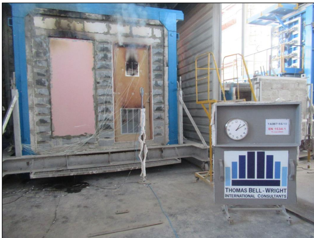
Picture 12: Unexposed face of doorset B after the termination of the fire test at 70:00 minutes.
