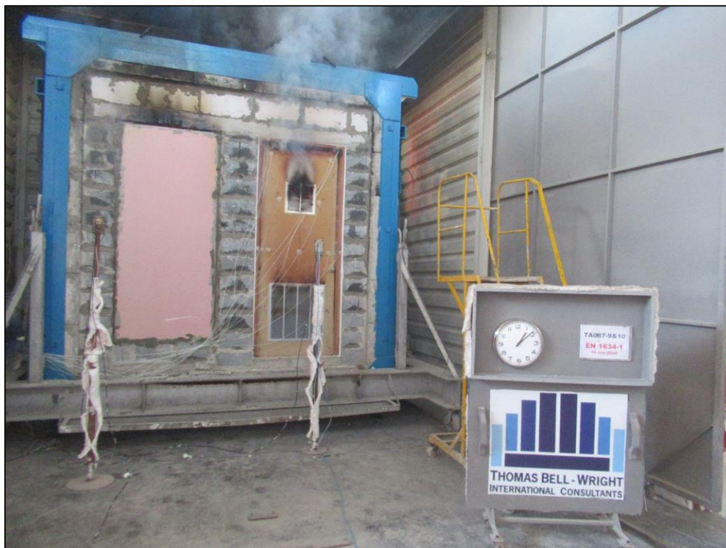
Picture 11: Unexposed face of doorset B prior to the termination of the fire test at 70:00 minutes.
