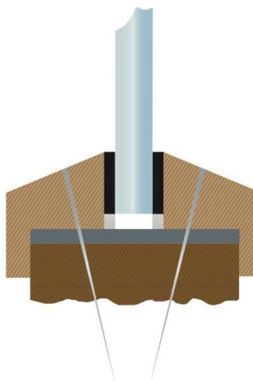
System may be used with and without non-combustible setting blocks. Care must be taken to ensure edge cover and expansion allowances for each specific glass are complied with.
