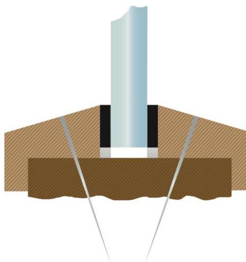
System may be used with and without non-combustible setting blocks. Care must be taken to ensure edge cover and expansion allowances for each specific glass are complied with. For modified toughened glass types (Pyroclear, Pyroswiss and Pyrotech 630) a minimum expansion gap of 5 mm should be provided.
